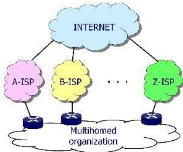
Fig. 1. Multihoming service provided by several ISPs
